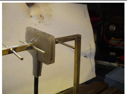
Shows feed point of the almost finished beam, tack soldered onto more brass box section for initial tests.
