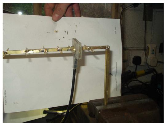
Shows the almost finished beam, tack soldered onto more brass box section for initial tests.
