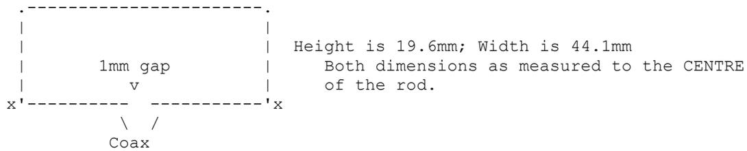
Bend the U first, get it spot on, then make the bottom as a single piece and solder it into the U at x. Now mark the centre and cut it through and file to a 1mm gap. The inner and outer of the coax then solder either side of the gap, as tight up to the gap as possible and with an absolute minimum of exposed core. The previously soldered corner joints need to be kept cool, to stop them unsoldering - I used wet tissue paper.
