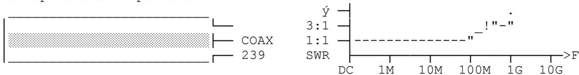
4/ By putting the resistive element rod into a conical box, the match can be maintained to much higher frequencies & the 1/4 wave problem goes away. UHF 100W loads are made this way.
