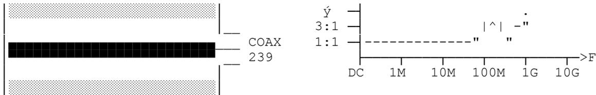
But they do suffer from 2 problems. They radiate at higher frequencies as the voltage on the outer is seen as a 1/4 wave & a good aerial, this also mucks up the load match. An outer cage reduces some of the radiation but does not help with the SWR.
