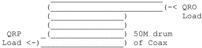
I have run >400W on 70cms on test this way without a QRO dummy load. The first few metres of UR67 coax did get quite hot though & there was some radiation, but the SWR was as good as you can expect from coax!
