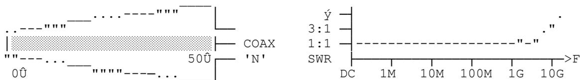
The internal load to conical box forms a coax, of the same Z as the load resistance element has left to go. The cone starting diameter is 2.3 (for 50Ω in air) times the rod diameter, tapering to the same diameters at 0Ω. The outer case may be a heatsink, but the hot resistance inside can easily be damaged by overloads.
