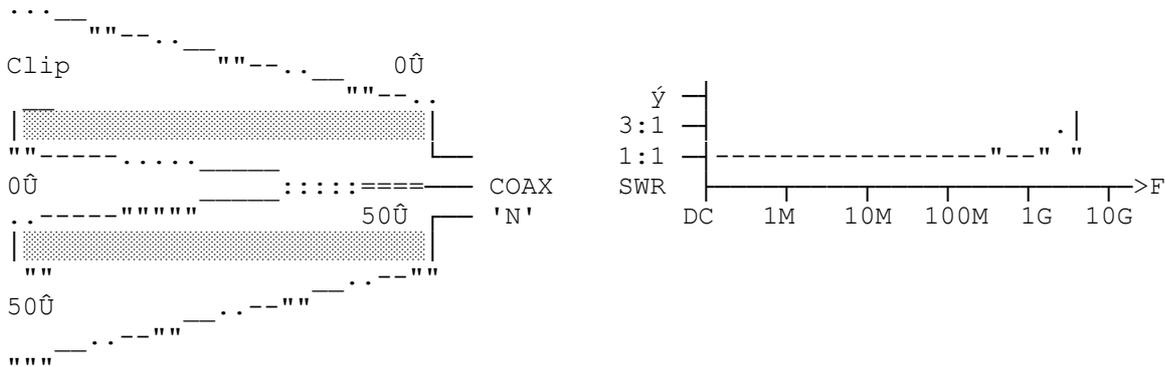
The inner cone is made from large coax braid soldered to a thick wire to the 'N' connector, & a clip holds the braid attached on to the outer of the ceramic tube end. The outer galvanised mesh (1cm holes) cone is bolted to the plate that has the 'N' socket bolted to it. The tube ground is by soldered on tags. There is some radiation with a mesh outer but dissipation is OK.
