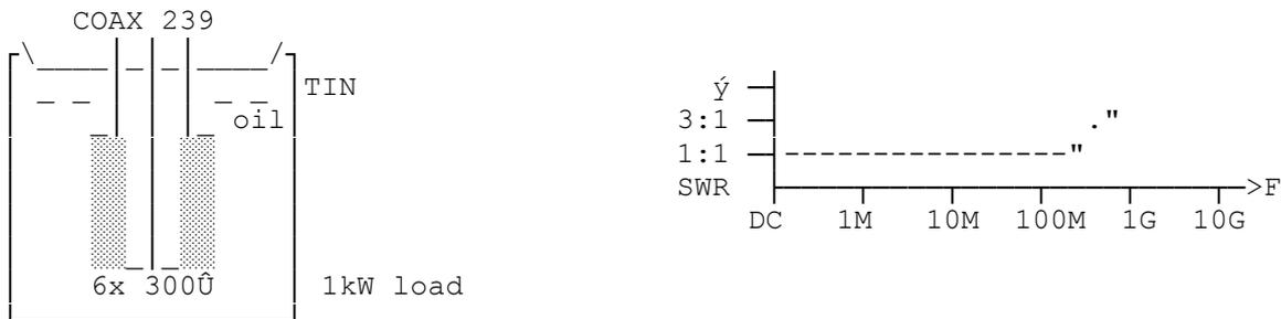
SWR limited to internal leads & large resistor size. Main problem with these is loss of oil through seals, or upturned tin etc.
