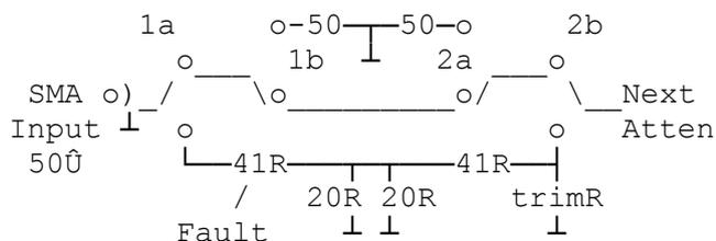
2 double change over relays 1 & 2 are used, this ensures high isolation with 4 contacts bypassing the through path when attenuating.
