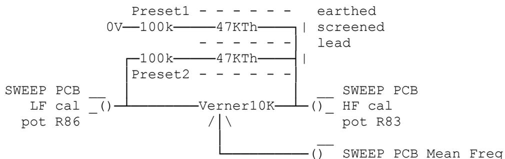
A thermistor & 100K Preset1 go to ground (Cal pot earth point) to the vernier tuning 10 turn pot most +ve lead (~5V), & 2nd thermistor with 100K Preset2 to the -ve of the 10 turn pot Vernier (~2V).
