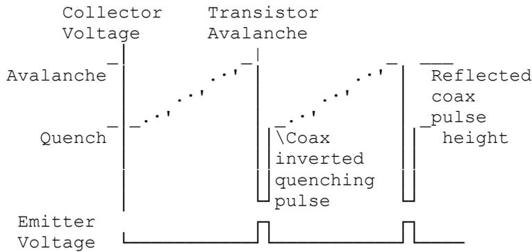
These can be used as they are, for coax cable time domain reflection testing with just a suitable T4 emitter network & a good oscilloscope. With a 14cm length of 50 ohm coax as the capacitor & very short wiring to the output socket, I found the pulse width was around 3nS wide [1].
