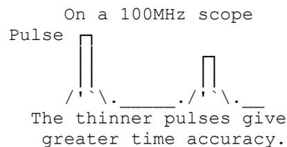
The location is the time difference between the initial pulse & the fault pulse, multiplied by the cable velocity, times 2 (there & back). Cables have velocity factors of between 0.66 of the speed of light (300M/uS) for solid coax, & 0.78 for semi air spaced types. Open balanced line velocity factor can be as high as 0.95.
