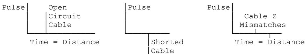
If the fault is intermittent or not extreme (not O/C or S/C), or an identical cable length is available, then a calibration of the scope can be done with the far end open & shorted representing 100% cable length. Then the fault location can be measured off as a % of that length, this can be more accurate than unknown velocity factor & scope timebase accuracy.
