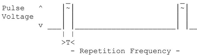
Due to the vertical sides of the pulse, there must be a spectrum null in the Repetition pulse frequency harmonics at a frequency of 1/T as a sine wave ~ could not fit in the pulse.
