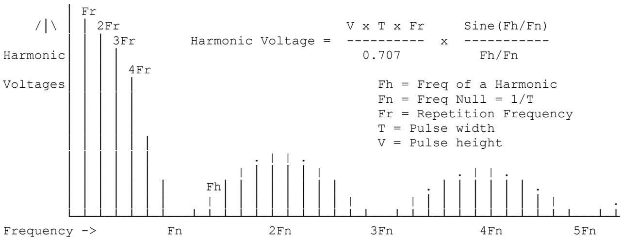
A spreadsheet can be loaded with this formula & pulse data, then graphs can be plotted of the ideal spectrum for comparison. This assumes perfect terminations & ideal pulse shape etc. but a good starting point.
