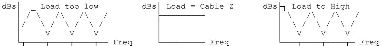
For short cables where the close in pulses merge, then the uneven spectrum ripple due to end mismatch echo on an spectrum analyser/scanner is then the best way to see matching, as it flattening out the frequency ripple when the termination is correct.
