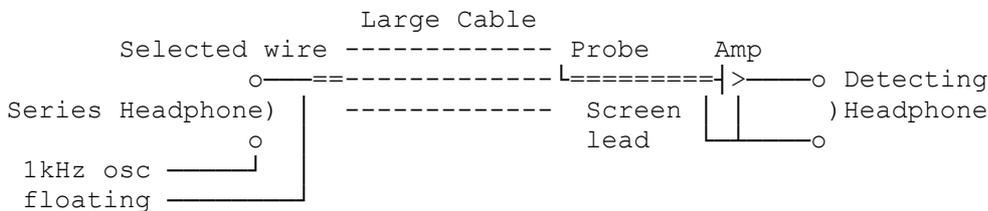
Here the cable is in audio pairs. When you hear the loudest tone in the detecting headphone from the cable, short that pair of wires together, & if the tone then goes, the send headphone gets louder, if not it is just a loud crosstalk pair (fault?) keep searching.
