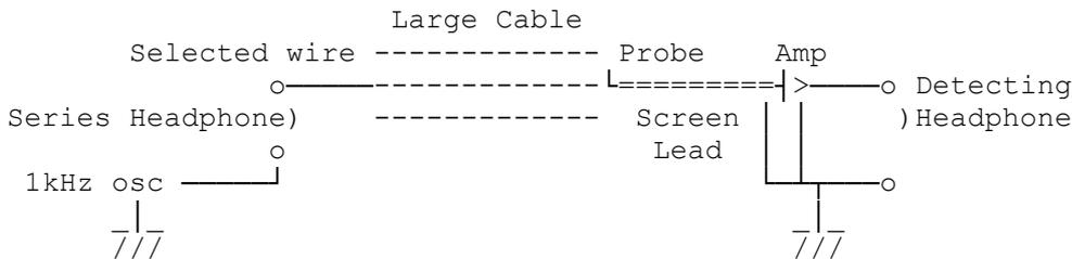
Here the cable is not in audio pairs, the return path is via earth. The probe is just an unshielded wire/rod connected to a short screened lead to the Amp. The Amp is very high gain (10,000x e.g. a 741) & tailored for 1kHz.
