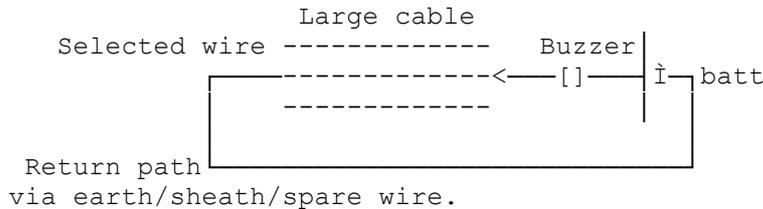
For in between connectors a Pin can be inserted into single wires to make connection to confirm the identity or prove the fault, but doing so will damage the insulation!
