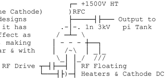
For large Tx valves the triode may even be run with no bias & very large amounts of Grid current, when the Grid is pushed positive by the drive signal, but the Grid must be designed for this, or it will be destroyed! In data books you see mode of operating "class A B or C" with suffix "1 or 2", 1 indicates NO grid current 2 is with Grid current.
