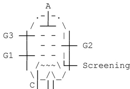
Variable gain (mu) can be obtained if the pitch of the G1 wire in manufacture is made variable, then increasing the -ve bias will slowly reduce the small signal gain of the valve rather than just cut off the whole valve. Rx AGC & Tx ALC use
