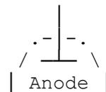
If the electrons are very fast then they can dislodge electrons in the Anode causing secondary emission from the Anode to other electrodes. To stop this some power valves use carbon/carbonised Anodes which better soak up electrons to stop most of this unwanted emission.
