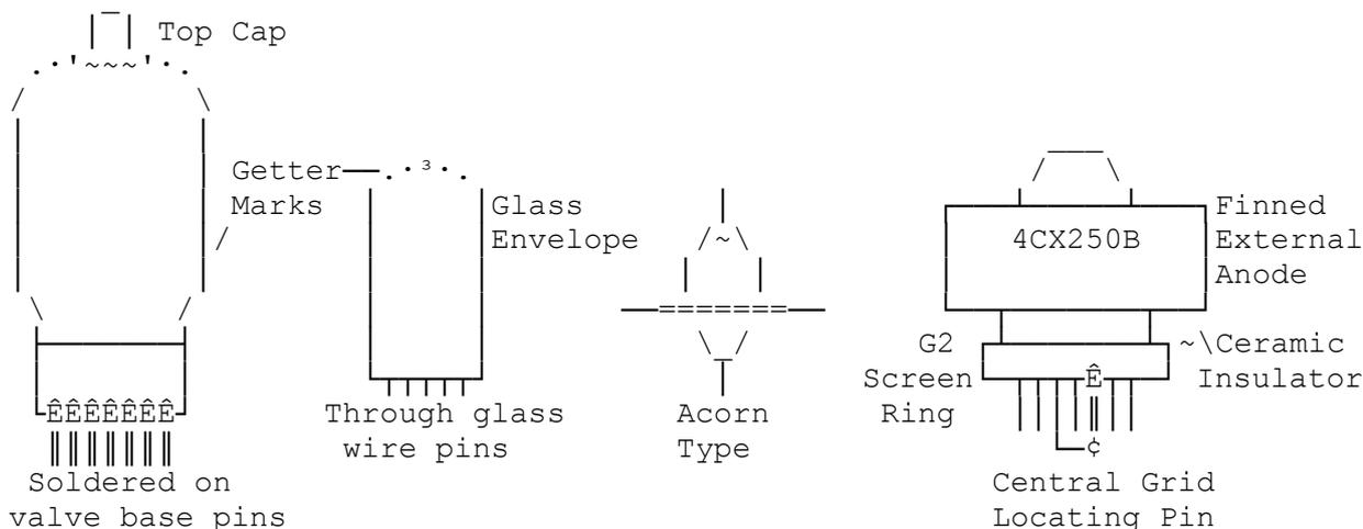
Many valves have top cap connections usually for Anodes on Tx & power valves like TV sweep tubes, but may also be a sensitive control Grid on Rx valves!
