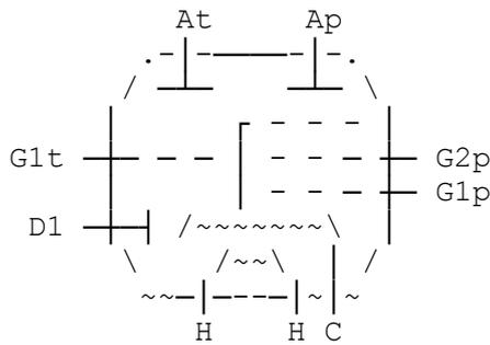
Some push pull VHF/UHF Tx valves use twin beam tetrode assemblies with one Cathode & G2, but two G1s & Anodes. Internal Anode to Grid neutralising capacitors between A'- G1 & A - G1' are possible with push pull valves in one envelope.
