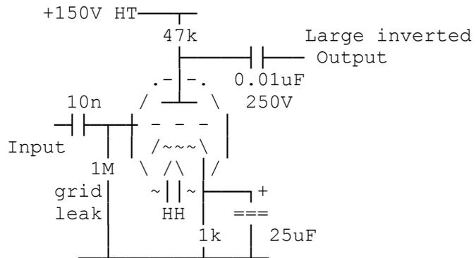
There is quite high capacitance between the Anode to the adjacent Grid & this causes high frequency negative feedback (Miller effect) in these high impedance circuits. The electron flow is proportional to the Grid voltage, but also the attracting Anode voltage, so there is considerable negative feedback in the triode, which keeps the Anode impedance low in common Cathode mode.
