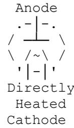
Unlike solid state devices, there is no voltage drop across valve signal diodes as the nearby Cathode electron cloud actually gives up electrons freely to the Anode (space charge current).
