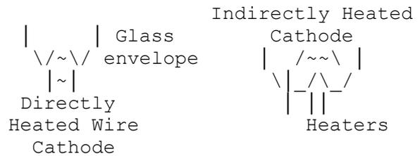
Directly heated Cathodes on AC supply often use a centre tapped AC supply, or a "hum dinger" pot across heater line to minimise hum due to the heater voltage.
