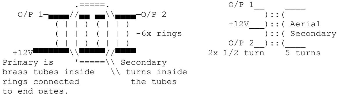
For higher frequencies & low power, bead types (miniature toroid), or double hole versions give extended frequencies up to 1GHz. The 2 hole one offers complex RF hybrid possibilities used in mixers etc.
