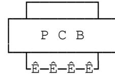
PCB mounts can be by soldering the connection pins moulded on to the plastic bobbin former.
