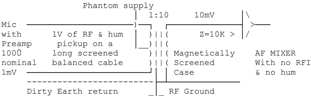
There are costs of course, as it is difficult to proved a wide frequency range needed for really super audio, but 40Hz - 15kHz @-1dB is quite achievable, with >60dB common mode hum & RFI rejection.
