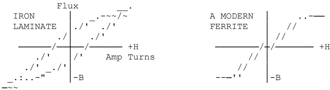
With ferrite the eddy current & BH losses are very small but have a sudden limit, & the BH curve magnetic cycle area which determine the power loss per cycle is also much smaller than for iron. (difficult to draw here).
