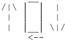
High circulating eddy currents flow around sides of large cross section like a shorted turn.
