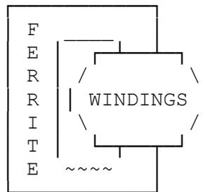
Maximum efficiency happens when the copper losses equals the iron losses.
