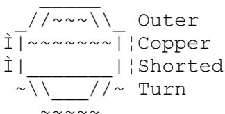
Further magnetic shielding can be proved by a copper strip around the whole bobbin former, but outside the laminations.
