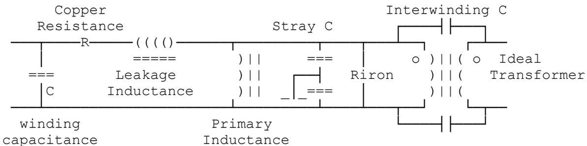
The iron losses are often indicated with "Riron" like this, but it represents both eddy current losses & BH curve losses, where the value is
