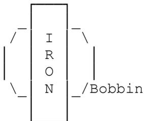
The weight of the transformer determines the energy through put for 1 cycle, so a 60Hz transformer is 20% smaller & lighter than a 50Hz one of the same rating. Ratings also depend on maximum safe enamelled wire temperature & the dissipation. E.g. a fan cooled one in a projector would catch fire without the fan!
