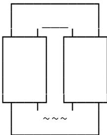
The core can be made from flat laminations or from U curved sections where each lamination is a different shape! In that case the magnetic flux leakage is much reduced.
