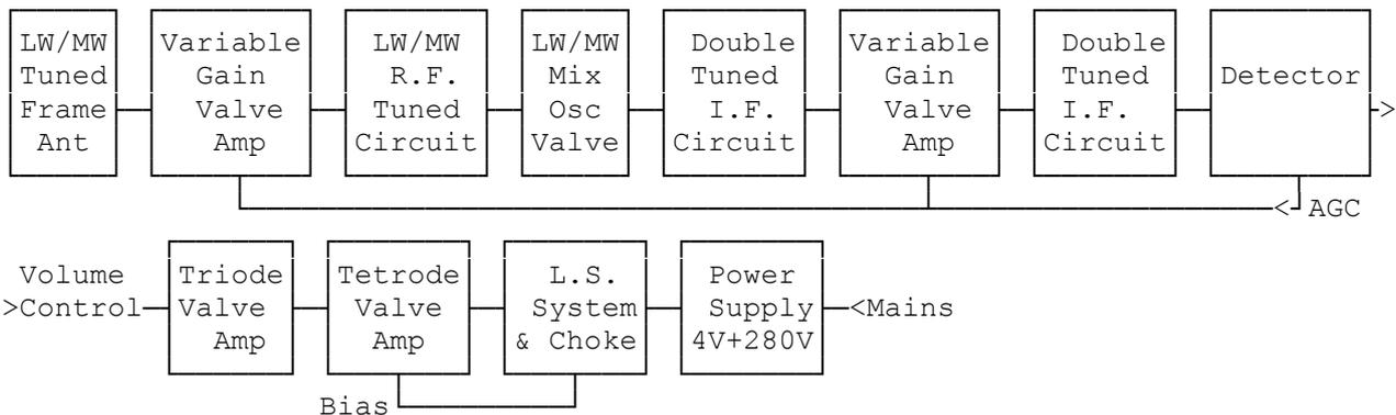
The detector is conventional double diode triode valve (MHD4) 7 pin, with high level signals from the IF anode used to generate the negative AGC line for the RF & IF amps. The AF detector feeds the volume control together with the Gram Pickup input & back to the triode preamp stage. This is coupled to the AF output. A leaky capacitor here, is a major cause of valve radios not working with the output stage taking all the HT power!
