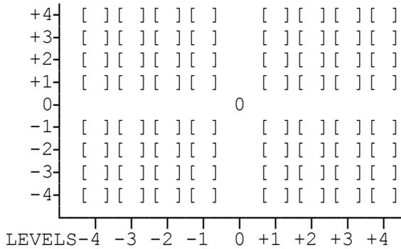
By using variable number of phases per carrier level, you can fill all the pigeon holes as close as possible, giving the biggest number of symbols, here 64, or 6 bits per Baud.
