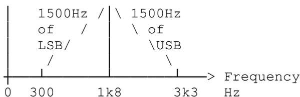
Alternating baud signals of 010101 @ 3000 baud forms the highest side bands of ±1500Hz.
