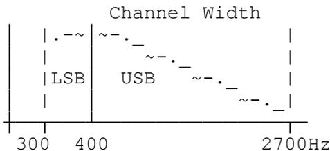
Only a tiny fraction of the LSB is sent enough to make the carrier in the linear phase & level part of the channel bandwidth. This gives the maximum Baud rate possible for any channel. BAUD is the changes per second, & DATA RATE is the number of bits per second. In single level AM, AFSK or FSK there is a 1:1 relationship, 1 bit/S = 1 baud.
