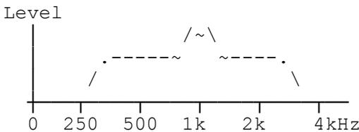
Add in a % of signal data from 500ms ago & the bump will go. But then you get a bump @ 2kHz, so add in some signal data from 250ms ago, keep doing this until all bumps are above 3.4kHz.
