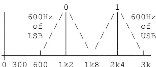
This is fairly typical of what happens as the FM idle carrier at 1800Hz causes 2 AM CW signals to appear at the deviation set points representing the data 0 & 1. Each of these carries full double AM sidebands up to the baud rate/2 in Hz, as it needs 2 bits to form a cycle. (1800Hz carrier is used as it is the fastest) (frequency on most telephone lines.)
