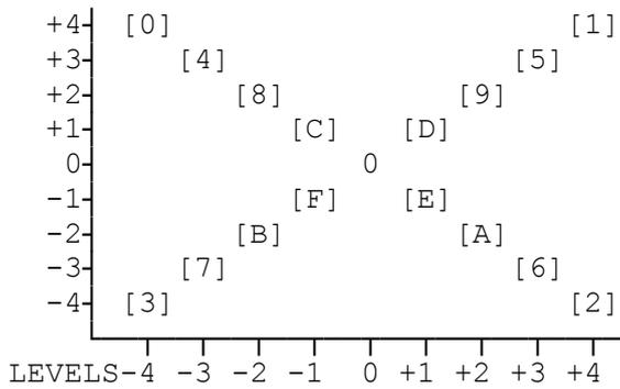
This give 16 pigeon holes (0-F) for each burst of carrier signal (baud) to drop into.
