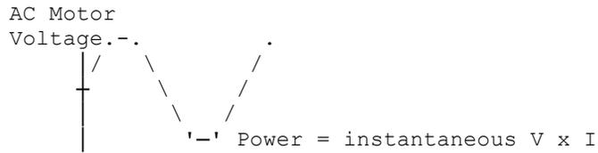
With modern true RMS meters & true AC power meter this can be can be accurately measured otherwise you are guessing!
