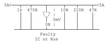
Or passing the safe current down the track or a bus, there will be minium volts at the fault site.
