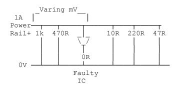
By passing a safe current of 1A via a car stop light lamp, this circuit will have voltage drop of a few mV down the +ve track. This will be seen as an increasing maximum to the fault then little increase after that.
