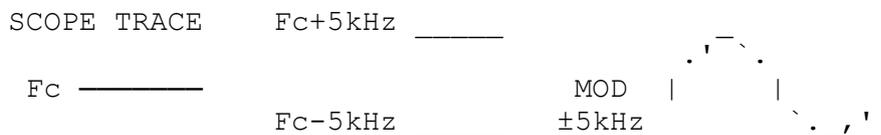
Send a carrier, & change the Rx/Tx frequency +/-5kHz & adjust the scope gains & position to give a +/- 5 division display.
