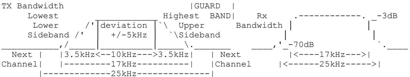
N.B. Here there is the luxury of an 8kHz GUARD BAND between channels on this system, which is why it can work much better with strong adjacent channel signals than the 12.5kHz system, & with very little distortion!
