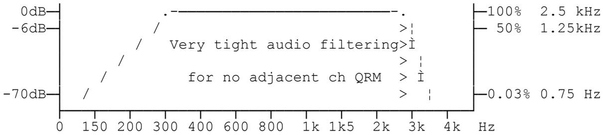
The ideal Rx IF filter can't be made (see Rx bandwidth diagram), so in practice narrower filters give better adjacent channel performance, but with quite high audio distortion (10%), as some of the needed spectrum is lost.
