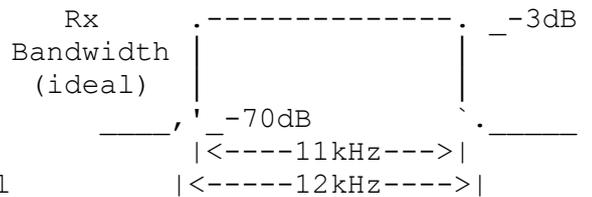
N.B. there is next to no Rx protection "GUARD BAND" between channels on the 12.5KHz system! For this reason commercially adjacent channels are NEVER used in the same area!
