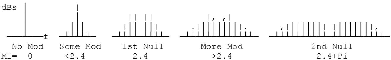
To monitor the modulation spectrum, you will need a SSB Rx with RF gain control, ideally with a very narrow CW filter, or a Spectrum Analyser with a narrow filter. E.g. a sound card from SSB AF output & an AF Spectrum Analyser programme, or just good ears listing to just the carrier whistles nulling while the other sideband ones get stronger.
