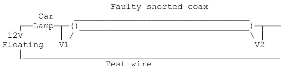
Here it is assumed the inner is OK & it has constant resistance per length. (if this is not true see "DAMAGED INNER" below)
