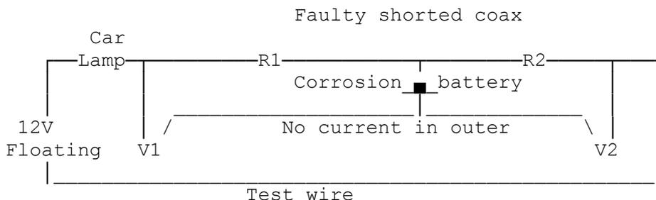
With a sensitive DMV measure V1 & V2, then reverse the 12V polarity & repeat. Average the readings at each end (ignore polarity) to cancel any corrosion voltage at the short.
