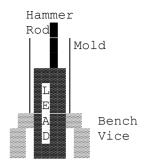
Holding the lead remains in pliers I heated them with a blow lamp & let them drip molten lead into the mold. When cool, I removed the steel plug, but found the lead was well stuck the mold. I hammed it out with the vice support just the mold edge.
