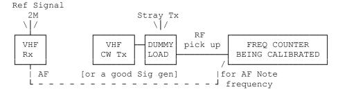
This assumes you have access to a Rx (ideally AM mode but FM/CW/SSB will do) that can Rx the beacon. And a CW Tx or a harmonic of one!
