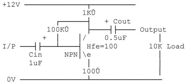
So in the above example Collector should be around +6V
