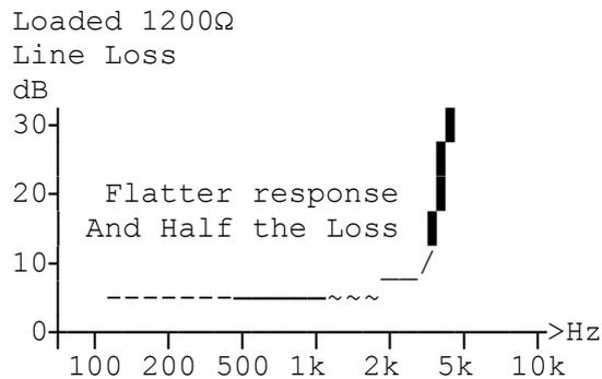
The standard for cables between telephone exchanges (office) was to use a loaded cable with an 88mH balanced coil every 2000 yards, starting 1000 yards from the exchange & completing the last 1000 yard pi section with a capacitor or a 44mH terminated inductor half section.
