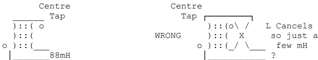
If just 1 winding is used then you have 22mH. By paralleling the 2nd coil you get half the DC resistance, but the phase must be right!
