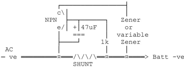
The transistor is a NPN. Make the shunt resistor (thick wire link e.g. 10-30cm of coat hanger wire bolted in place as it will get hot!) so at the maximum current wanted it drops 0.6V, enough to make the NPN conduct, & hence reduce the zener voltage & thereby limit the current. The 1k & 47uF filtering is needed so that the average current is controlled not the high peak current.
