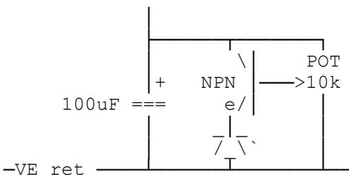
The Zener can be 5-10V (12V system). The transistor is an NPN. Set the voltage
