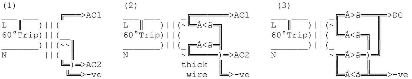
The transformer must deliver an RMS voltage slightly greater than the battery voltage plus diode & wiring losses. If voltage too low, triggering the SCRs can be difficult. Tn that case use an additional 2V winding put around a toroidal or leg of the transformer to feed the trigger circuit can keep the unit working well on low mains (the train PSU had to deal with mains of less than 200V AC at times).
