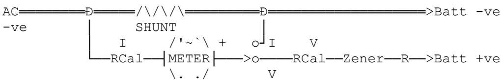
Leaving the I RCal preset in line on voltage measurement will produce a small error, but simplifies wiring. Calibrate the V & I meter scales with external meter, adjust suitable presets for full scale. In the voltage case an additional fixed series R (e.g. 1k) can stop meter accidents! Also a 10V zener in series can give a more useful offset scale e.g. 10-15V.
