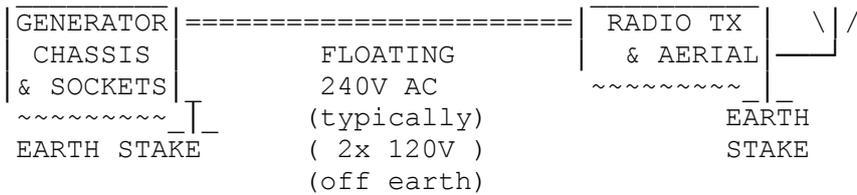
With actual balanced supplies 120-0-120V where the 0V is hard grounded (e.g. 110V building site transformer) there is still a shock hazard, but much reduced. But the current from either side of feed needs fusing, or you could do welding to earth with it!
