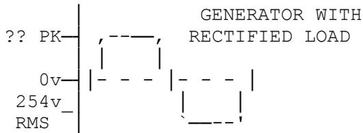
So to partly remedy this, some over voltage is desirable, say 253V, the mains maximum. But at this voltage resistive loads like lamps & valve heaters will have reduced life, but the HT or PSU headroom will be a little more like normal!
