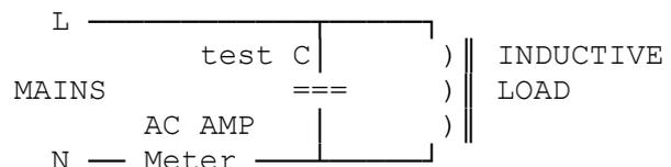
The exact amount of C needed to tune the load can be measured if you have a bank of suitable caps to try out. Use a an AC Ammeter in series with the N wire to the load & try out various Cs in series/parallel until you find the value needed for minimum current. Warning mains is dangerous & caps stay charged!
