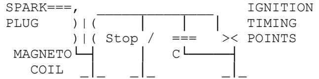
The points are arranged to open a few degrees before "Top Dead Centre", when the magnets are also across the coil. When the points open the magnetic flux is allowed to enter the coils, & soon produces a powerful decaying oscillation with the condenser.
