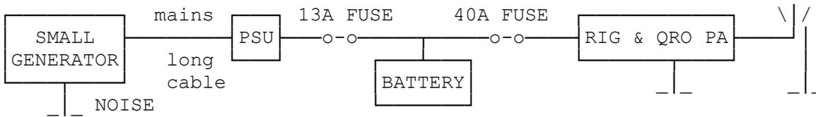
Also ensuring that no Tx station sharing a generator, has to run full carrier power for tuning up valve PAs, so by use "werlos" (not whistles) & PEP METERS. This can solve excessive mains dips on heavily loaded generators enabling several 400W SSB stations to be run from a single 1.5kW peak rated generator.
