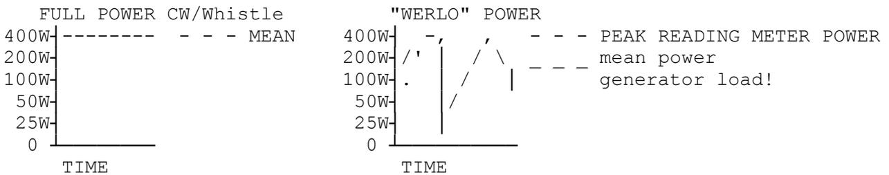
e.g. a 400W station needs at least 800W DC input (class B or AB2 valves) for full carrier tuning up, but only 450W DC for spoken "werlo" 400W PEP tuning up.
