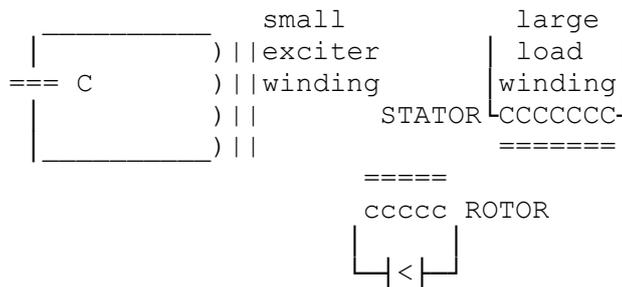
On starting the small residual magnetic field in the rotor produces a 90° leading current in the capacitor & self exciter winding. By transformer action this produces a voltage pulse across the diode in the rotor & charges up the rotor's magnetic field. As the rotor spins this occurs twice each revolution.
