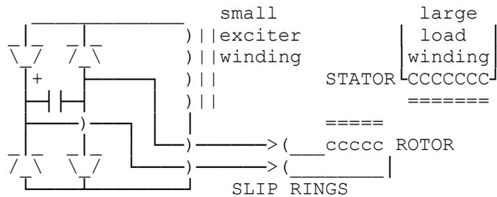
On starting the slight magnetic field left in the rotor is enough to overcome the bridge rectifier loss to enable the excitation to build up the rotor magnetic field. Sometimes to aid quicker excitation, waste engine magneto power can also be added with another diode.
