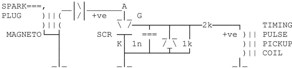
Electronic types replace the points with an SCR that suddenly shorts out the magneto +ve voltage as the magnets pass. Some use a separate induction timing pickup coil & small magnet on the crankshaft produce a precise timing pulse, resulting in the sudden change in the magneto primary winding voltage & the secondary then produces the high voltage. Ignition kill system on low oil is also common.
