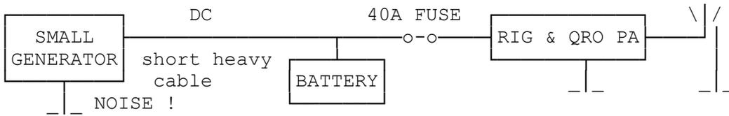
A 200W SSB Tx needs 35A peak, & regulated 10A PSU will be able to cope with that provided is well rated. But this is not so good for high power FM, but the battery will still recover on Rx.
