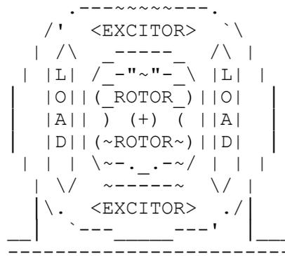
If the rotor is shaped correctly & the stator windings are evenly spread the rotating magnetic field will produce a sine wave in the load winding. But this is not the most efficient use of materials, so cheap efficient single phase generators often do not produce a good sine wave waveform!
