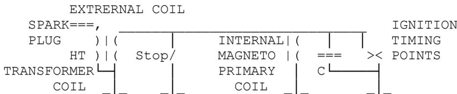
A second high voltage coil (that can be an external ignition transformer coil), produces 15-25kV to power the spark plug.
