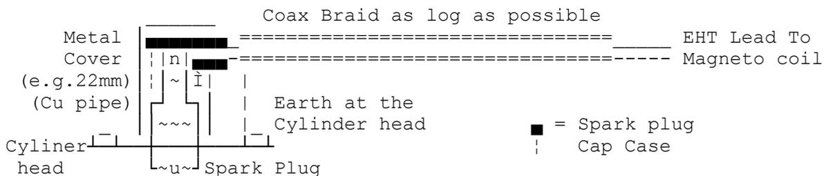
Suppressing plugs & screened caps are also available, but resistive lead as used on cars is not normally possible due to the magneto lead connection.
