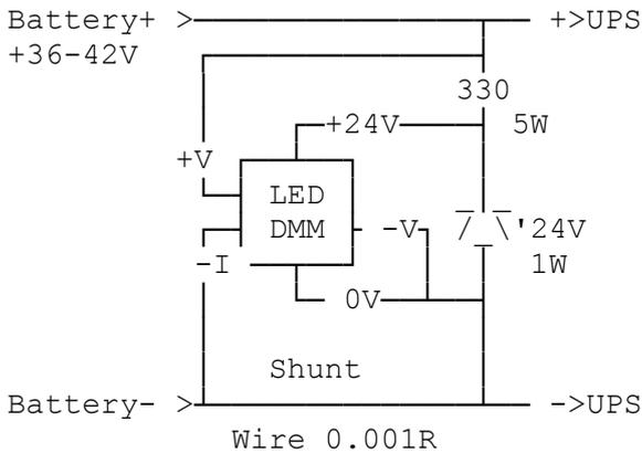
The current shunt only needed a few mV, so the voltage drop across 1ft of thick wire to the rear connector was more than enough I calibrated it (preset pot) with a 10A load & DMM.
