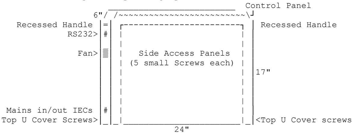
After removing the steel side panels, the top steel U cover comes off with 3 plug leads.
