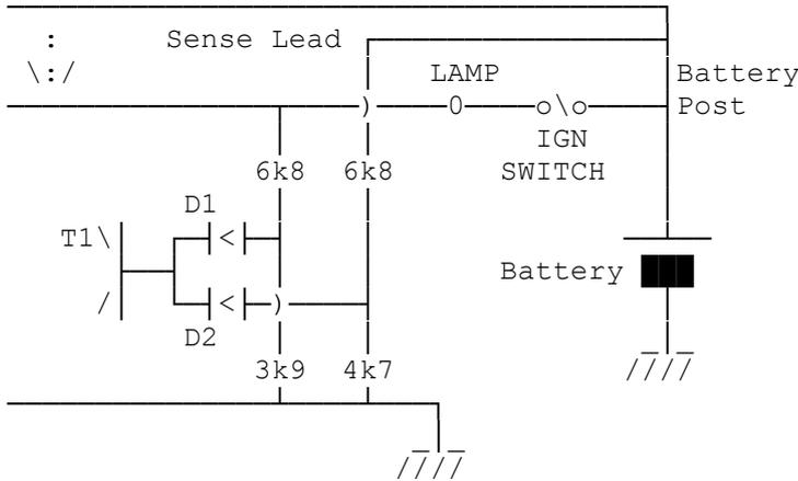
There are 2 attenuator samples, the normal internal exciter's voltage, as well as a lead sending the actual battery voltage. The 2 attenuators are slightly different permitting 14.5V on the battery terminals or 16.9V on the internal sensor.
