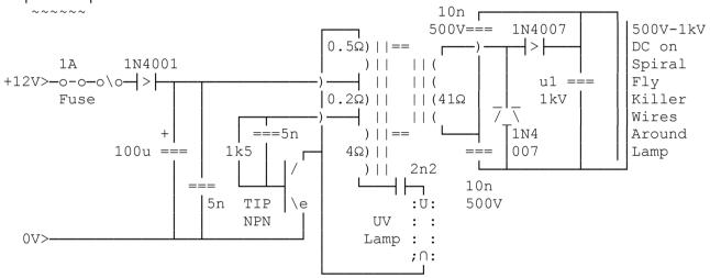
It uses a standard E ferrite transformer core except there are two bobbins one on each end rather the one in the middle. This magnetically isolates the high voltage fly killer circuit & it can be shorted out or not without affecting the UV lamp inverter much.
