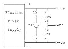
The asymmetrical currents & voltages will affect the components needed (e.g. transistors have to handle peak offset current & heat), in some applications, e.g. value of 1K R may be 39K on 100V. Higher currents may need darlings or P & N ch MOSFETs.
