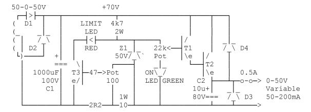
T2 2N3055 on a heatsink, or other 100V 50W NPN TAB or MOSFET instead of T1 & T2 T1 & T3 BFX84 or other 100V 500mA NPN
