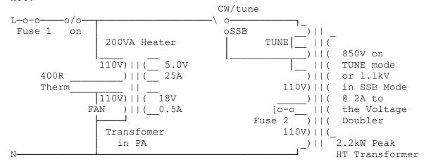
Results were the heaters now take 3 sec rather than 1 sec to warm up now, filement volts dropped a bit from 4.9V to 4.6V. But RF power still 900W max on low power setting HT tune setting. So the heaters are bright (hot) enough!
