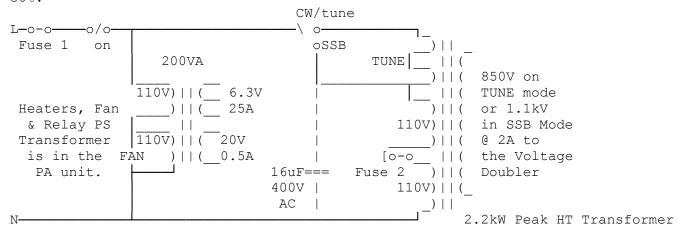
For 110V mains, all the windings are put in parallel not series.
