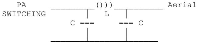
For 2M C=23pF & L=1-3 turns 1cm dia to give a SWR 1:1 match into a good load.
