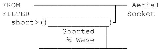
Start with slightly longer piece of coax than a ¼ wave x coax Velocity Factor. e.g. 48cm. Tee this across the aerial socket & leave open circuit. With a good aerial & Rx connected, cut down the coax length a bit at a time to null out a Rx signal. Check the null is good with the coax in it final position (around the PA etc). Then without shortening the coax make cut into the inner insulation & solder up a short circuit.
