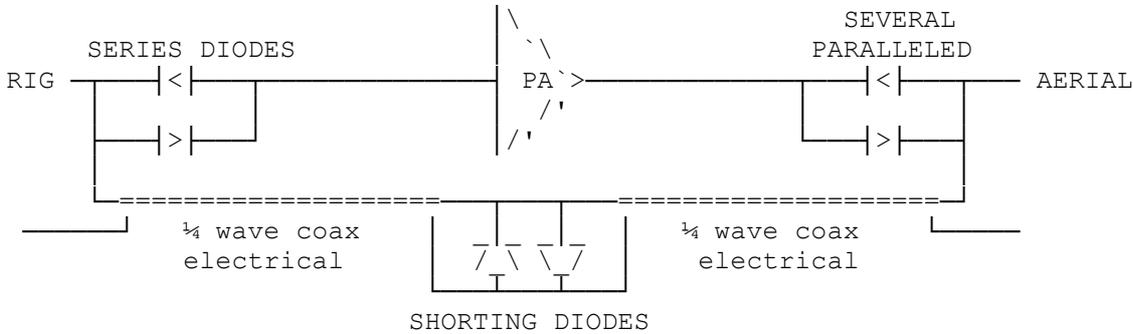
This is the standard circuit. RF Diodes (1N4184 or better) connect the PA when the drive is > 600mV & drive the aerial through diodes as well, these may need paralleled diodes for > 10W. In Tx the Rx path is short circuited by the diodes a 1/4 wave from both the Rig & aerial, therefore presenting high Z to both.
