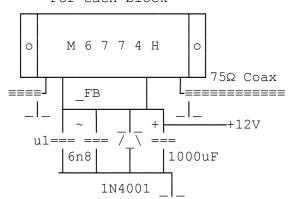
Power filtering capacitors are applied to each module keeping the leads short for good VHF practice. A ferrite bead is used to feed DC1.
