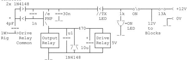
A tiny amount of drive RF current is fed through the 4pF to voltage doubler to turn on the PNP (\* I tried different values & this worked with my PNP & relay load @ low drive power OK). The 2 change over relays are both plastic encapsulated ones, the drive one is a smaller 5V DIL type, they are both held in place with a local earth tag soldered to the coil connection & the coaxes ground there too.
