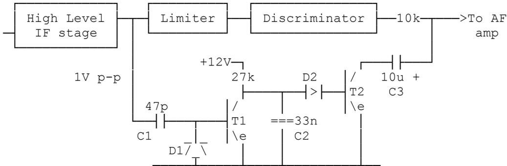
It works on a 600KHz IF in my application, so I expect the circuit will work on most 455KHz IF systems without too much of a tweak. With a scope I first checked there was a pre limiter stage with enough IF level to drive a transistor stage into class C, if there was not I would have added another IF amp to raise the level, as it happed I was lucky large signals to work with.
