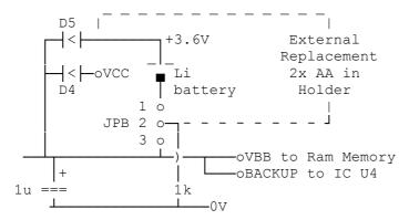
As you see from the circuit there is very little other than the 1uF protecting the static sensitive memory IC from external electrical shock (static & HF). The Li battery current limiting 1k earth resistor left in the external battery system only making matters worse!
