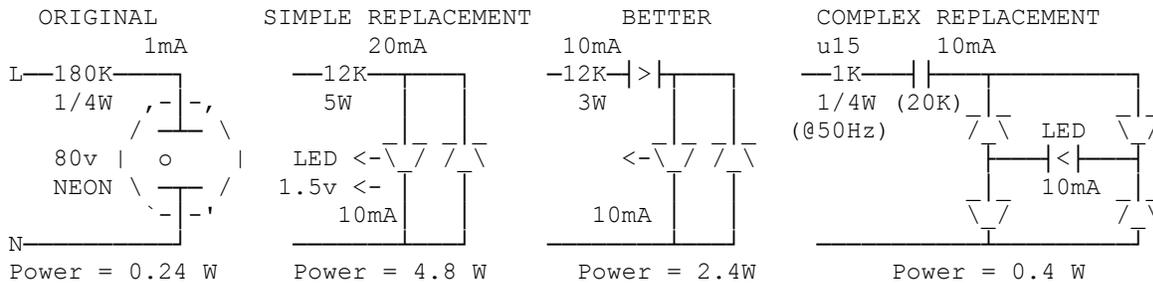
The Neon has 80V drop & to give reasonable brightness 1mA is needed. Whereas the LED needs say 10mA @ 1.5v drop for the same sort of brightness as it is far more directional light source. 100Hz flicker (50Hz 3 each end).
