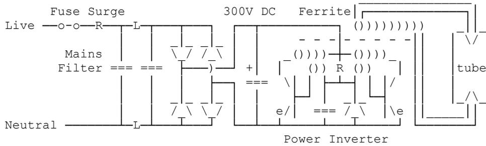
The mains is protected from the large HF inverter QRM by the mains filter. The Surge R has to handle turn on surges (>340V peak). The always live 300V DC is roughly filtered by the electrolytic cap & the supplies the high frequency current path needed by the inverter. Here I have shown a simple push-pull high power inverter, some use driver control ICs & MOSFETS etc.
