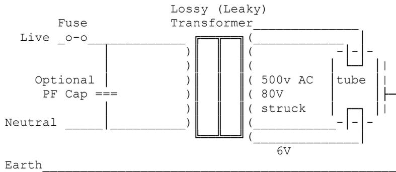
These use either a non resonant lossy transformer with a magnetic shut that allows the flux to bypass the secondary. (An isolating one is shown here but auto-transformer types are common). A resonant transformer with a series tuning capacitor, this can cut down the size of the transformer while also correcting the PF.
