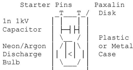
When the starter contacts cool down, the contact breaks & if there is still mains current flowing (not at the wrong part of the mains cycle) high back EMF from the choke is applied via the mains across the tube. If the tube fails to strike the start cycle repeats.
