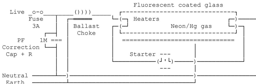
The ballast choke is designed to give the correct heater current (1A) when the starter shorts & also give the correct arc current (lamp rating) when running. The capacitor is optional depending if the mains power factor (due to inductive ballast) needs to be corrected, & even then usually only to a PF of 0.85-0.9.
