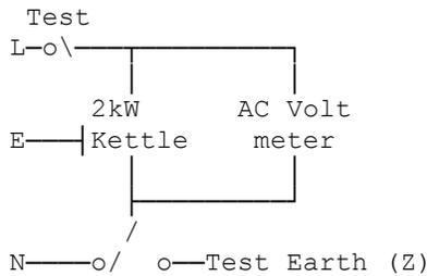
This high current & voltage test overcomes some of the errors of low current & voltage testing due to corrosion etc. As direct mains is involved some basic safety needs to be considered. And if you have just filled the kettle are U wet !
