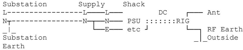
Now suppose the Neutral is not at ground, say 100V off ground due to unbalanced load 3 phase loads or someone is blowing a fuse. The 100V now sees your path to earth as an alternate rout to the substation. How many amps can your rig take from aerial to PSU & PSU mains lead? None of this is fused all can just burn out/catch fire!
