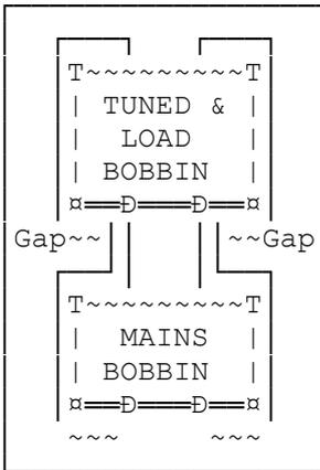
Specially shaped transformer laminates.
