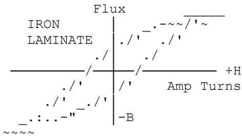
The BH curve shows the magnetic flux B saturate & flattens off as the magnetising effort in Amp Turns increases. This is the heart of the regulation principle.
