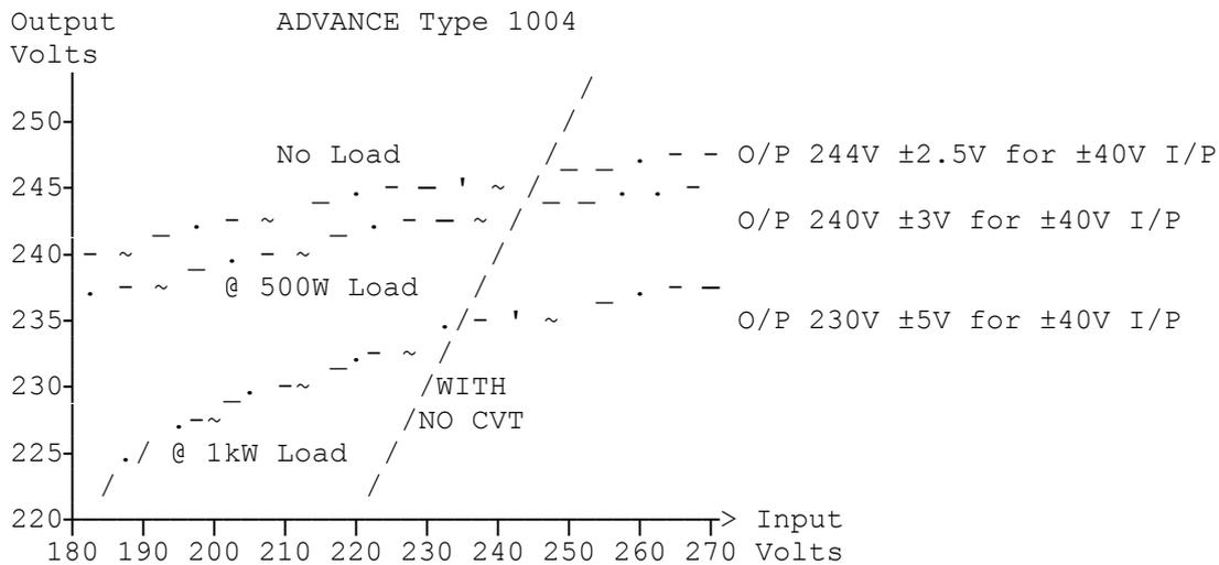
The regulation only occurs of course at the resonant frequency. The output is a fairly low distortion sine wave but not that good. Note that the output rapidly drops with the heavy overload, & in fact overloads tend to give a fairly safe constant current at just over the maximum current rating.
