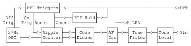
Features include an LED showing PIP tone is armed (lit during Tx overs) & a "K" LED showing the K leaving.
