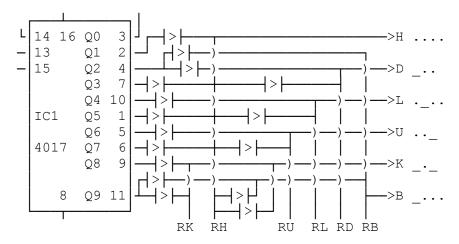
A multi way logic selector etc, to select the letter before the AF osc to give... No modulation = no CW, K = OK, B = On Battery Power. L= Low Mod, H = High Mod, U = Freq Up, D = Freq Down, all depending on Modulation & FM Discriminator DC output etc..
