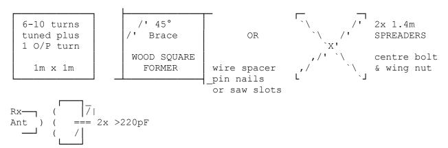
The exact number of turns depends on the L you end up with, its inter-winding capacitance, the frequency wanted & the tuning C used. An alternate to more turns for LF end (LW) is a switchable 1000pF cap teed across the tuning C.
