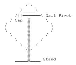
The turns used was 8 + 1 secondary. I did not use a taped coil as this unbalances the tuned circuit making it more susceptible to near body interaction.
