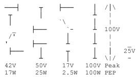
The carriers can be at any phase angle, on 4 different frequencies & quadrature phase angle modulated, but at some time the vectors will all add up in phase.
