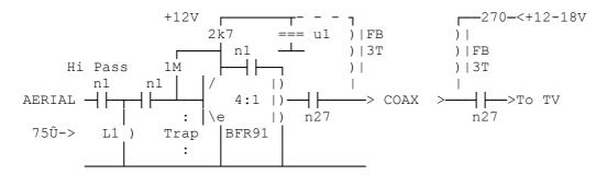
You can power this one from local 12V, the 2k7 & 1M are supposed to bias the transistor to 2.5mA for minimum noise maximum sensitivity. But higher gains & more linearity can be achieved if you change the bias as needed..
