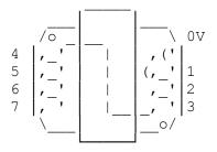
Adjustable connection is made with a small wander crocodile clip to the linking straps. Typically 2-3 of the 7 taps gives the best for the  $80\hat{U}$  headphones. Mount it well to the base board (e.g. 2 screws tapped into the 4 plastic corners not near the winding!) as it is heavy component.
