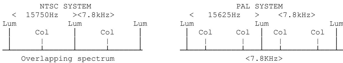
But the PAL alternate line inversion (7.8kHz) of the (V) colour vector, ensures there is NO phase error (colour hue) seen in the signal. Like NTSC there is also minimum, but some interference to the luminance especially on fine diagonal patterns when the sidebands will clash.
