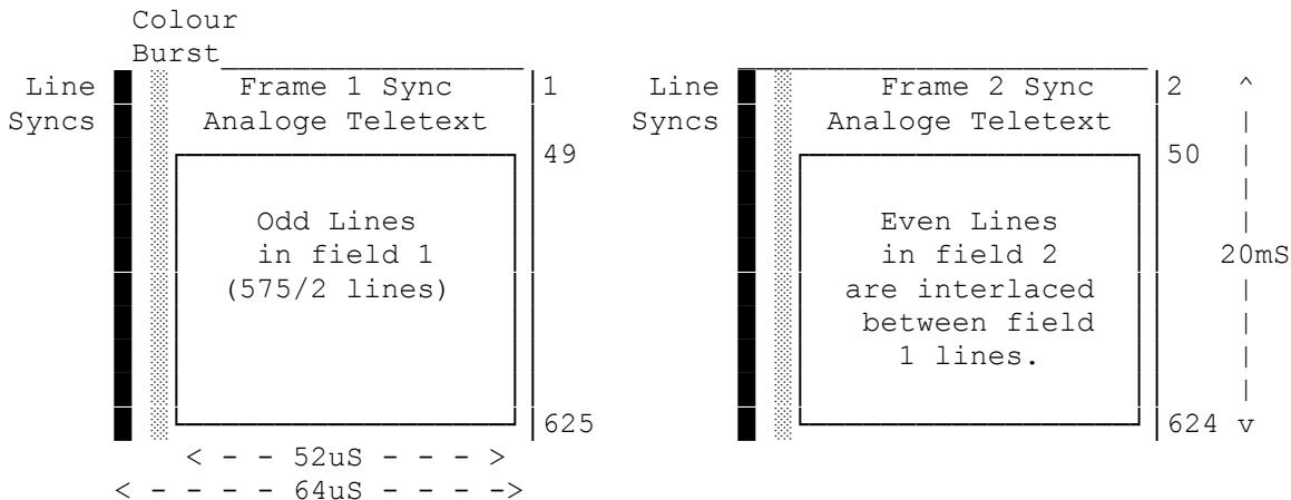
The 625 line interlaced system actually has only 575 lines of picture. 50 lines is taken up with the frame Equalising pulse, frame pulse, teletext & or blanking lines.
