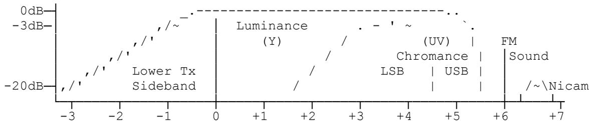
As you can see the luminance (Y) bandwidth 5.25MHz @ -3dB which at 52uS per visible line gives a 500 lines of infinite precision analogue horizontal definition. e.g. A vertical line edge (pixel) can in any position.
