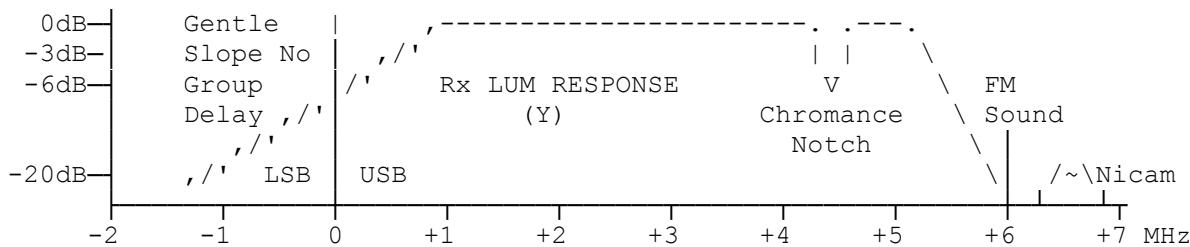
The recommended -6dB 400kHz wide Colour notch, used to be applied in the video stage to reduce fine chrominance patterning in strong colours, enabling the otherwise full luminance bandwidth to be used. Because there is some delay in extracting & processing the PAL colour signal a luminance delay line is needed.
