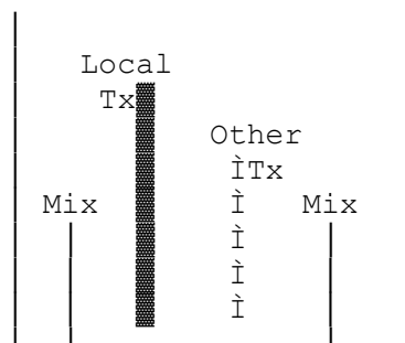
Aerial Port Spectrum Showing External Mixing (mix bigger than Tx Port)
