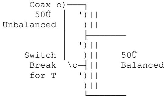
The transformer losses/SWR were bad & the Marconi T mode, just disconnects the earth, & so it did not drive the dipole equally & left some of the inductance in series.
