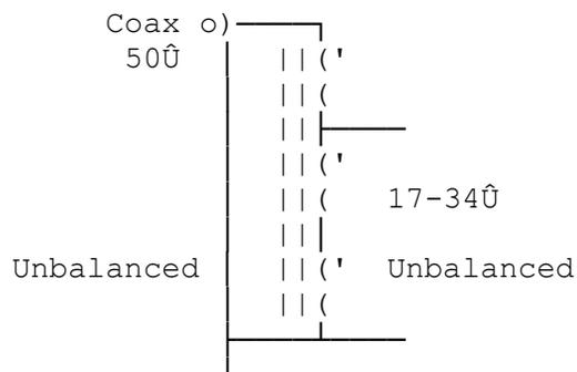
9/ 1:2 Auto Transformer. 1:4 Z (uses 2 windings)
