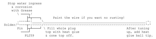
To solder to galvanised steel is straight forward with some solder fluxes, if not with yours you will have file the wire to provide keys for the solder to grip the wire. If using stainless steel wire rod, heavy cross keying with a hacksaw will be needed to achieve any physical grip with normal solder.
