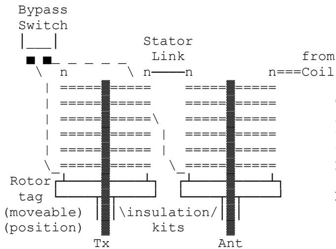
The shafts should have been at Tx & Aerial voltage & never the high voltage (kV) end of the power tuned circuit! Even though there are plastic front shafts for the knob brass sleeve & screws etc.
