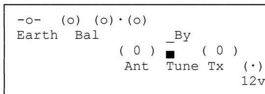
It is a small cheaply made unit, the 2 tuning Cs are "preset types" with only 1 bearing, so they will soon short out with wear or by a dropping on their knobs!
