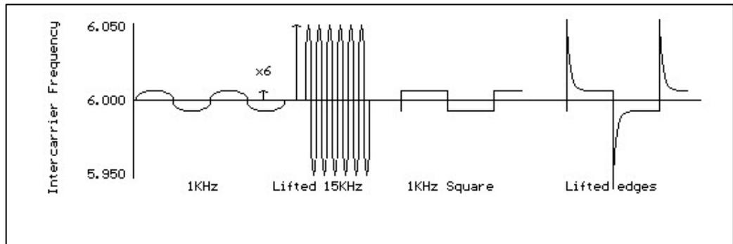
connected!). First set frequency to 6 MHz, then put the scope probe on the output of the preset deviation control. Connect up a pot (1k-100k) across a supply rail & use the DC on the slider to swing the opamp's bias up & down, & hence the Varicap DC high & low.
