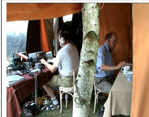
LH John G8MNY on HF RH Mike G3TWJ on LF with K1 QRP transmitter sending and receiving morse code (CW)
