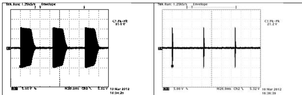
**Figure 13** Waveform at Q308 collector as the synthesizer is approaching lock while adjusting the **Synthesizer Tune** control from the high frequency side left. Waveform at Q308 collector when the **Synthesizer Tune** control is adjusted away from a nearby lock point.
