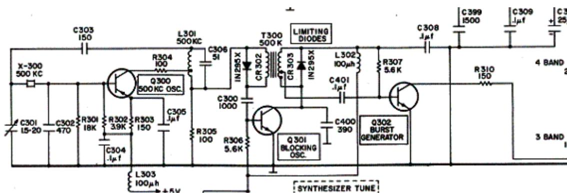
**Figure 2 Synthesizer harmonic generator**
