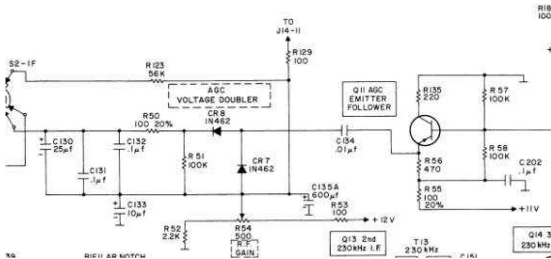
If this AGC section of the radio has any problems it can drastically affect the apparent sensitivity of the receiver. Test this circuit by applying dc power. The voltage on R53 will be about 11.3Vdc since there is a protection diode in series with the dc power supply input. Now check the voltage on C135A. That should be at 8.9V, if it's much higher, then R52 has probably changed value and shifted high.
