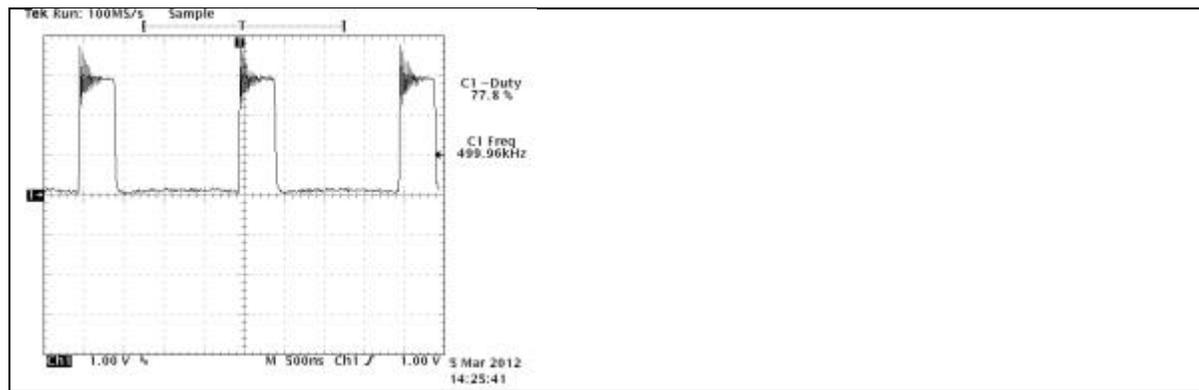
Figure 8 Q302 burst generator collector waveform
