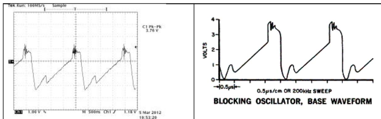
**Figure 4 Q301 blocking oscillator base waveform as measured, left, and as illustrated in the manual as Figure 22, right.** Note that the manual illustration does not show the actual dc offset of the base waveform but does represent the amplitude correctly. The actual waveform has a large negative component due to the base conduction on positive peaks.
