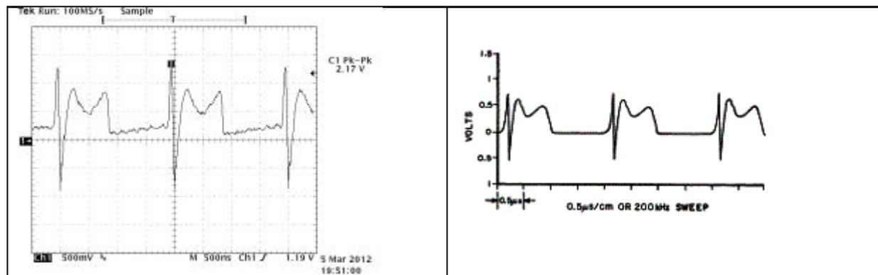
**Figure 3 500kHz oscillator waveform as seen at R305, left, and as illustrated in the manual Figure 21, right.**
