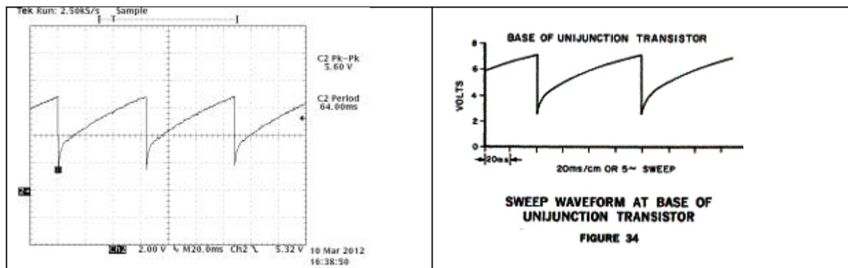
**Figure 14** Waveform on the left is at the base of Q311 when the synthesizer is not locked. The sweep period illustrated is 80ms.
