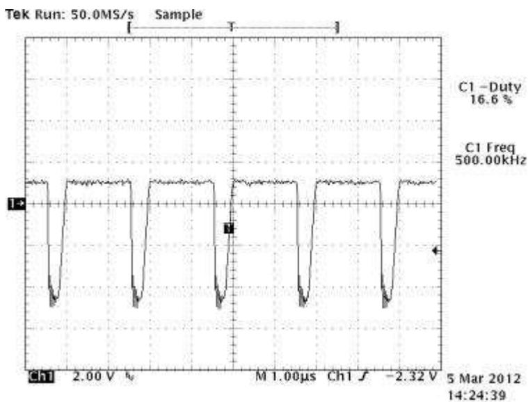
**Figure 7** Q302 burst generator base
