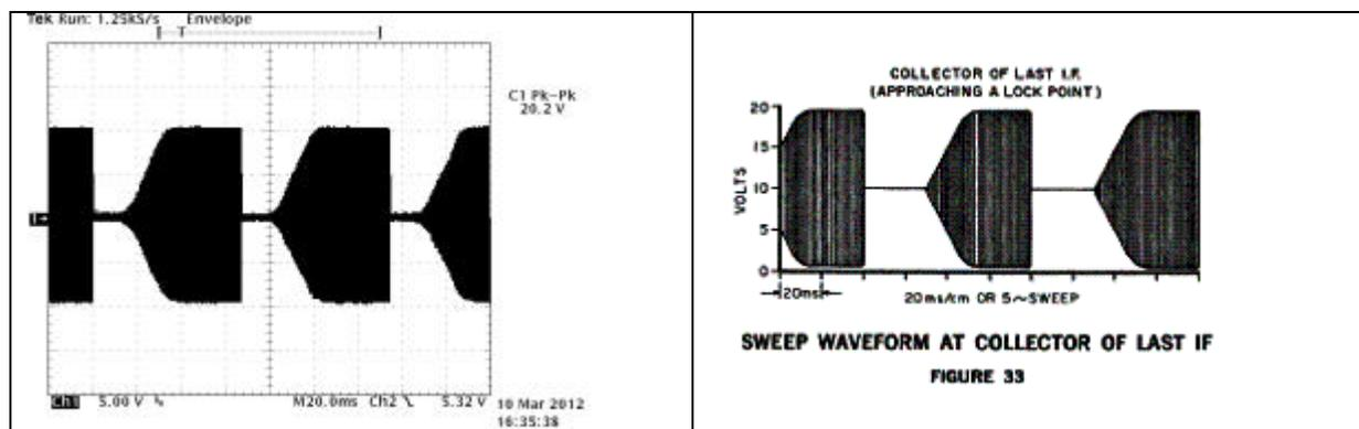
**Figure 12** Q308 collector waveform as the synthesizer is approaching lock while adjusting the **Synthesizer Tune** control from the low frequency side. Actual measured on left and illustration from manual on the right.
