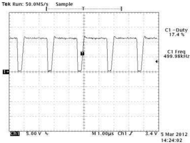
**Figure 6** Q301 blocking oscillator collector normal operation
