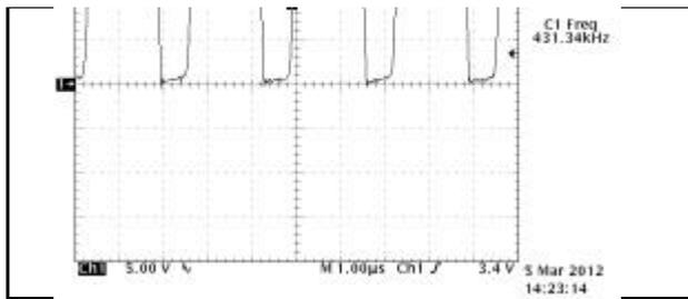
**Figure 5** Q301 blocking oscillator collector with 500kHz crystal removed. Notice that the free running frequency is 14% lower than when the blocking oscillator is synced to the 500kHz reference oscillator. This is normal and a good check of the blocking oscillator operation.
