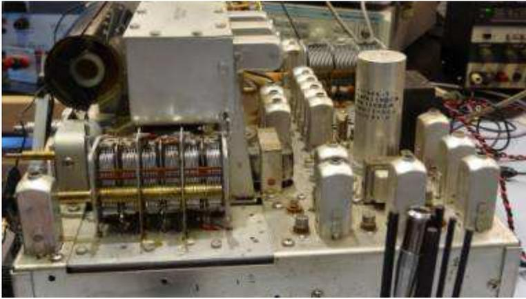
**Figure 1 Passband tuning six-section variable air capacitor shown with shield cover removed in order to align the plates**
