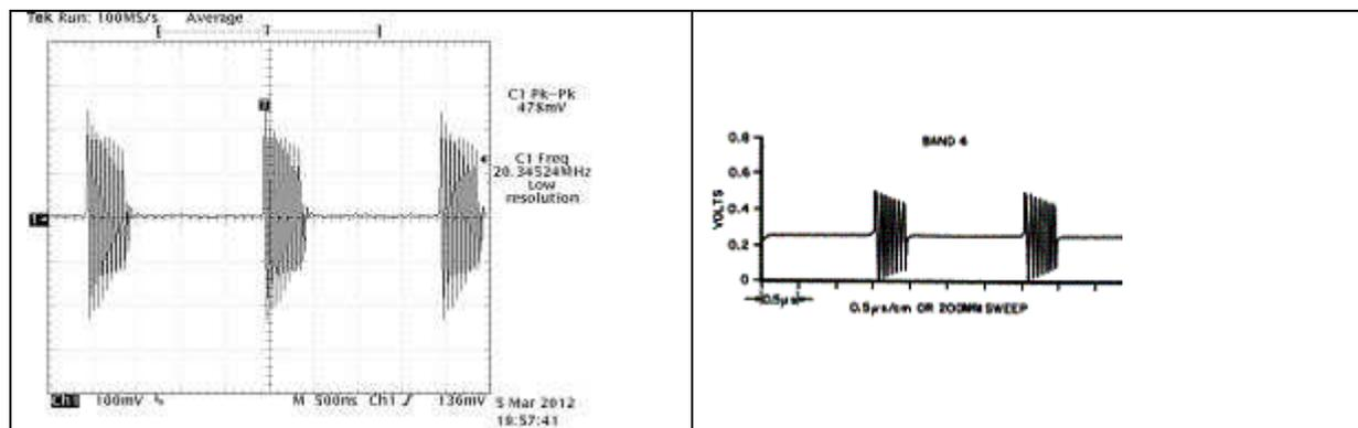
Figure 10 Spectrum generator output for Band 4 as seen at junction of C345 and C346, left, and as illustrated in the manual Figure 24.
