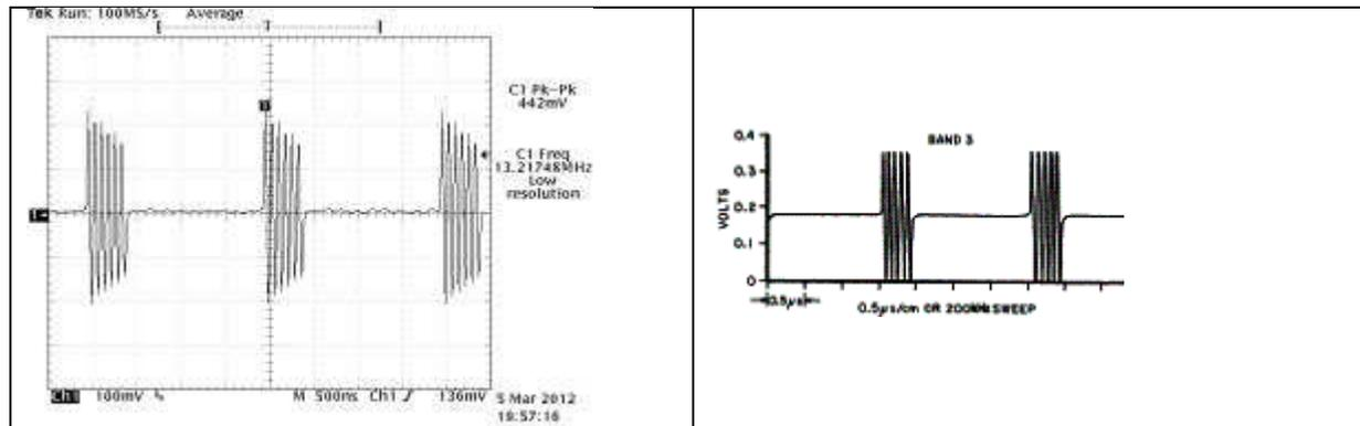
Figure 9 Spectrum generator output for Band 3 as seen at junction of C345 and C346, left, and as illustrated in the manual Figure 24.
