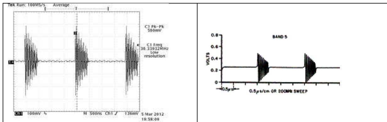
**Figure 11** Spectrum generator output for Band 5 as seen at junction of C345 and C346, left, and as illustrated in the manual Figure 24.
